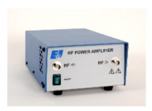
The 403LA Broadband Amplifier is a rugged source of RF power suitable for a variety of UHF signal distribution and general laboratory applications. It is a compact fully solid state design. It features low-level intermodulation distortion and inherent protection against short and open circuit loads. The 403 LA amplifies the inputs of AM, FM, SSB, pulse and other complex modulations within its output and bandwidth capability.
